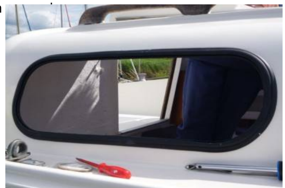
New Window Seal Fitted
