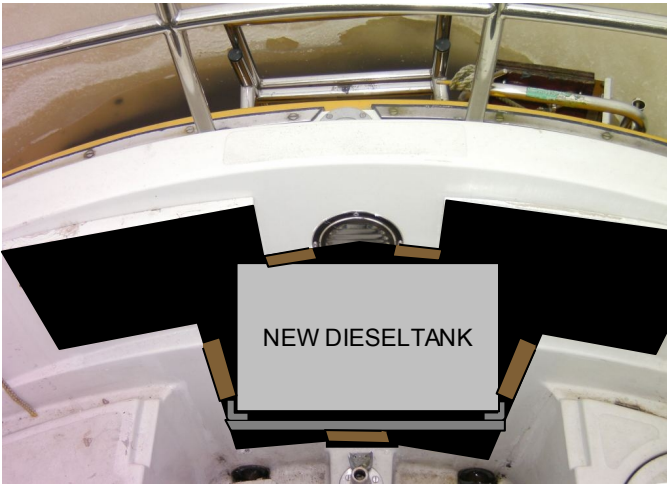
PLYWOOD SUPPORT RIBS LAMINATED
