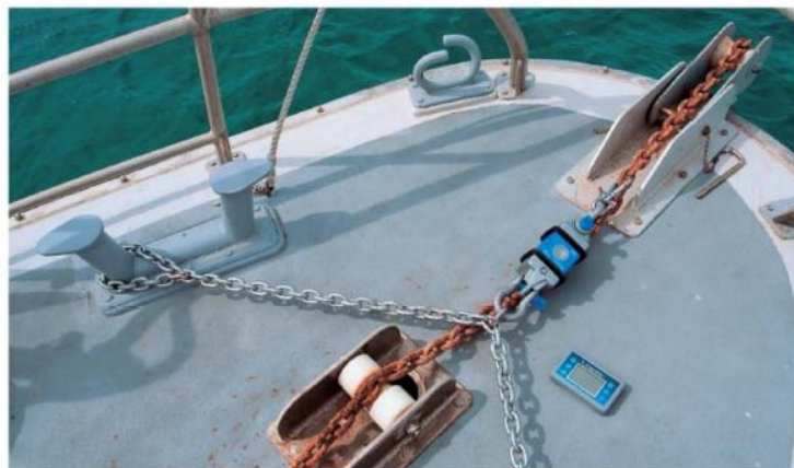
The lifeboat's bulletproof bow roller enabled us to exert more than three tonnes of force on the anchor cable, and measure the cable loads accurately with the dynamometer
