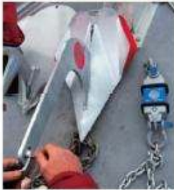
The dynamometer recorded the force on the cable every hundredth of a second
