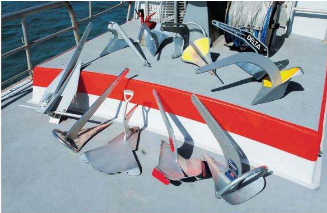
The anchors we tested were all of a similar size, but with a wide variety of shapes and surface area
