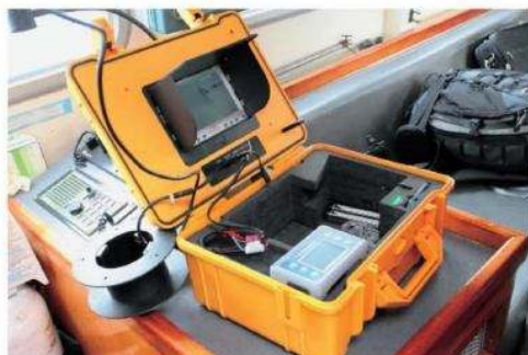
The elaborate test rig enabled the team to see live data from the dynamometer while they watched anchors setting and breaking out
