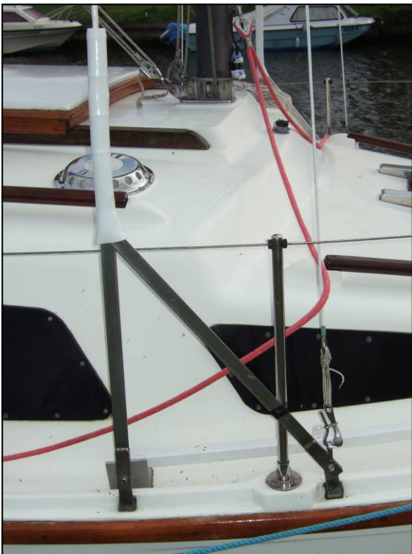
Fig 5: Shows triangulated shroud bars which bring the pivot point for the cap shroud in line with the pivot of the mast.
