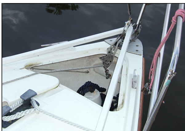
Fig 1: Shows A frame tackle secured to an eye bolt in the anchor locker which was screwed into the stiffener piece which is moulded in the bow of the Leisure 20.
