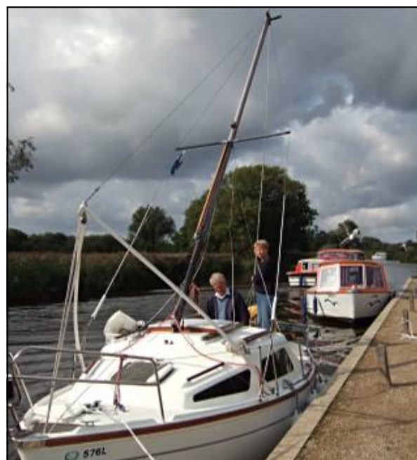
Fig 2: Moment of lowering the mast - you can see the tension retained on the cap shrouds.
