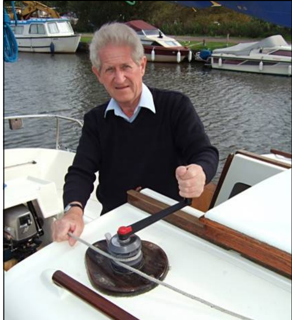
Fig 6: Shows the small self tailing winch on the cabin to, (already on the boat when purchased!) which we use to raise and lower and gives complete control during the operation - this is not compulsory as there is enough advantage in the lowering tackle but it does enable both of us to stand in the cockpit and allows us to stop and start the movement of the mast at any point - it also makes the whole business a one handed operation if need be!
