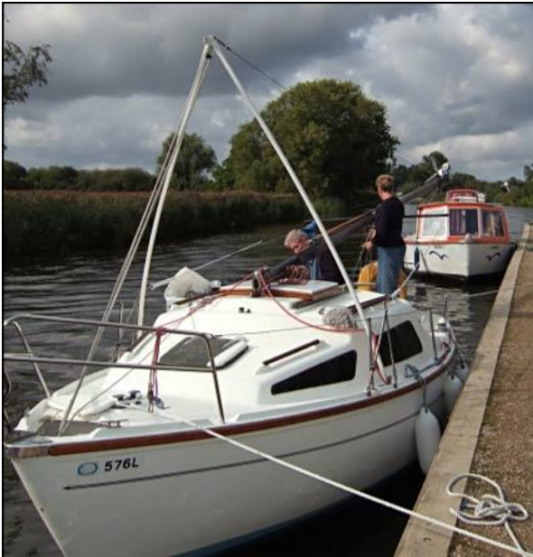
Fig 4: Mast lowered and resting in mast crutch at the stern (this crutch is a permanent structure on our boat).
