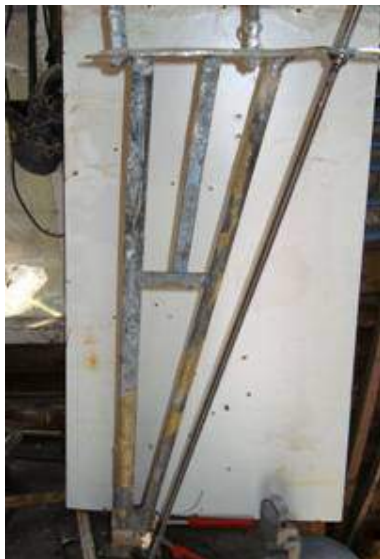
1): Useless bolt removed and new threaded rod added
