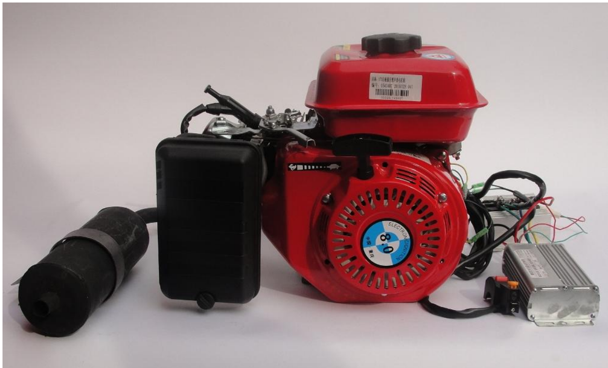
After assembling fuel tank and flexible exhaust
