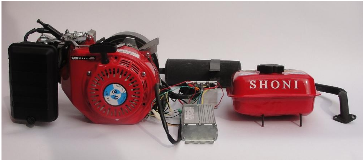
Left to right: generator with carburettor and air filter, electronic controller, fuel tank and flexible exhaust in the back
