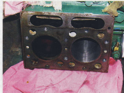
Only forward cylinder bore has been honed so far
