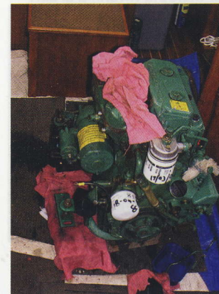
Reassembled engine, note slot in mounting plate and rag tied round fuel pump banjo bolt
