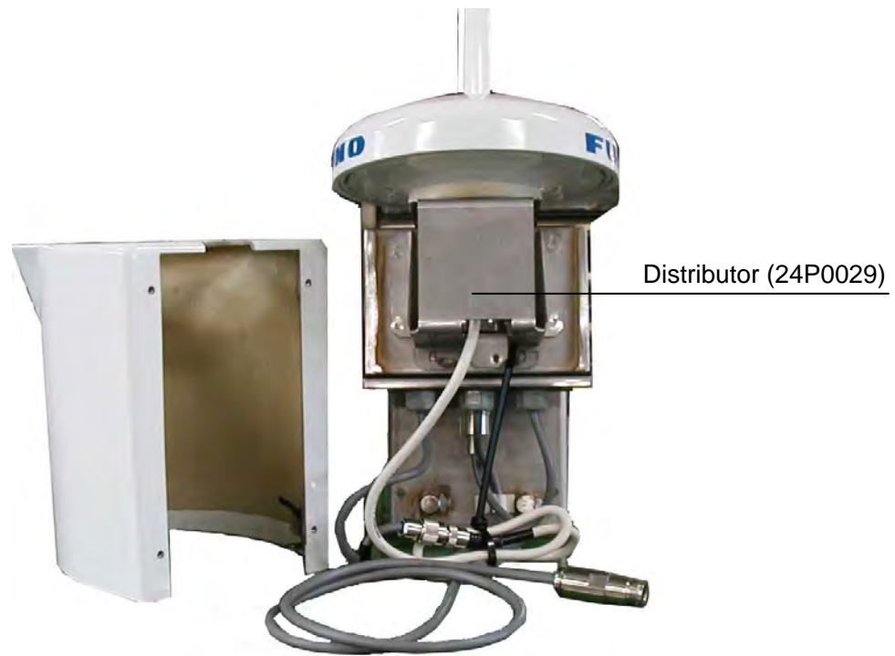
Figure 3.2.3 GAV-100 with the cover removed
