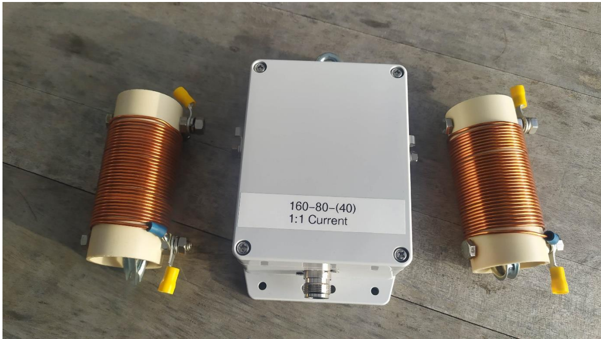
Figure 2: similar 23uH coils and a current balun as used as well in the dual band dipole design
