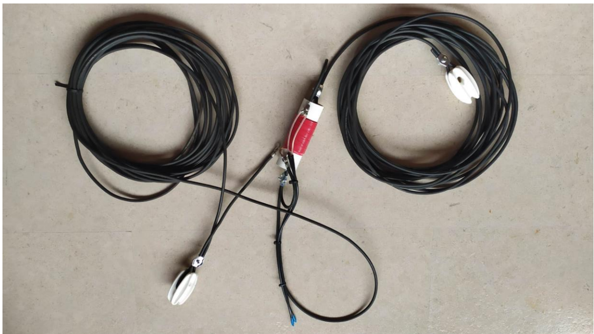
Figure 3: a picture of a dual band vertical using the non-resonant trap principle. The tuning capacitor is mounted in parallel with the wire side coming from the balun, grounded at that side so there is no extra inter-wire capacity. To decrease length I used two pieces in parallel. Ends are slightly stripped and insulated (blue tape) to prevent arcing in rainy weather.
