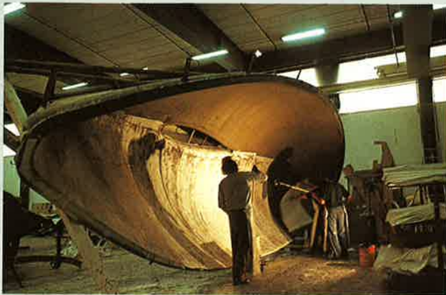
Handlaid glassfibre – a disappearing art these days.
