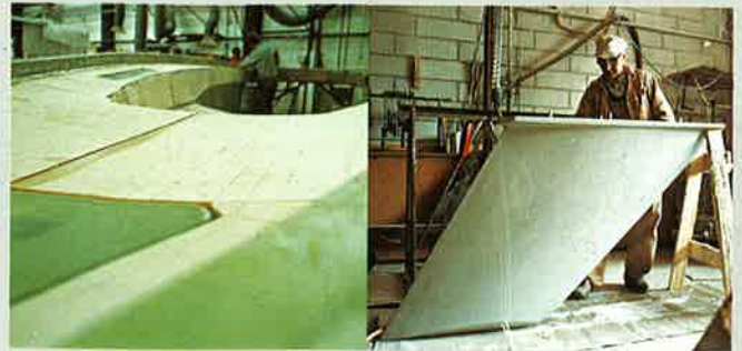
Full sandwich construction on all horizontal surfaces. The keel – an alloy of iron and lead cast in glassfibre. Something else you don’t see every day...
