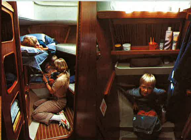
Forward cabin. Locker on the left. Toilet on the right. The toilet doubles as a shower cubicle. With teakwood grating.
