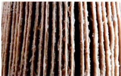
Filter blockage due to high Cloud Point
