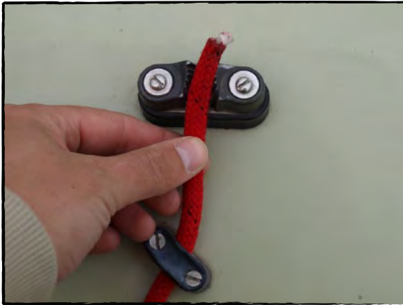
Photo 13, Pass the jib sheets through the jammers
