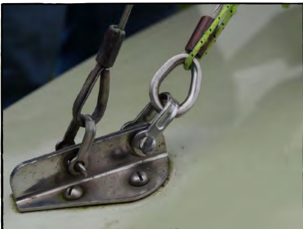
Photo 8, Attach the jib to the chainplate
