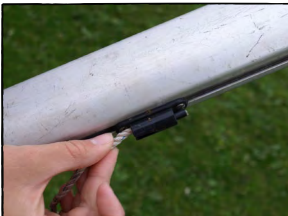
Photo 17, Feed the outhaul rope through the cleat
