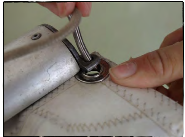
Photo 16, Pin the tack of the main sail
