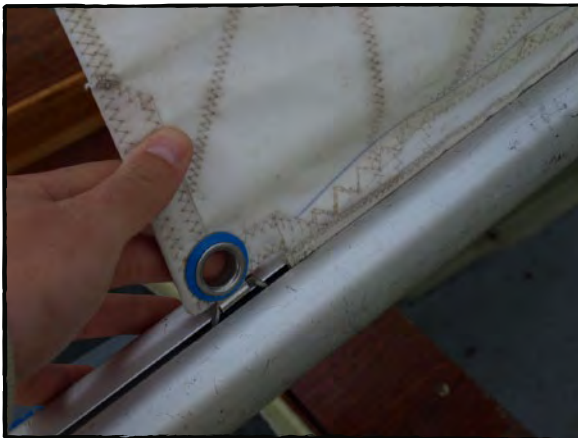
Photo 15, Pull the main sail along the boom
