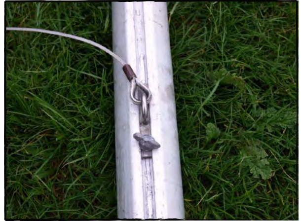
Photo 7, Kicker attachment on boom
