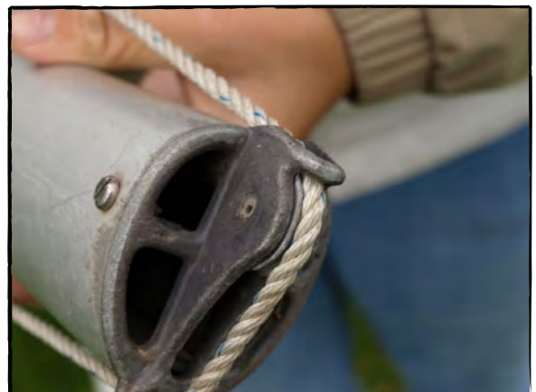
Photo 18, Pass the rope around the boom end
