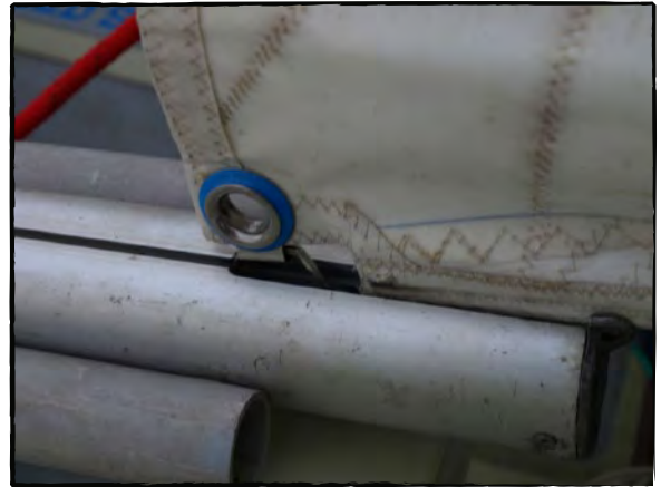
Photo 14, Put the main sail foot car in the boom
