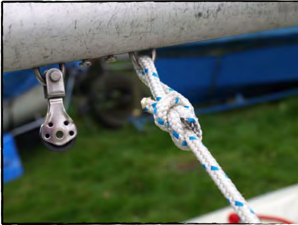
Photo 32, Attach main sheet to the boom
