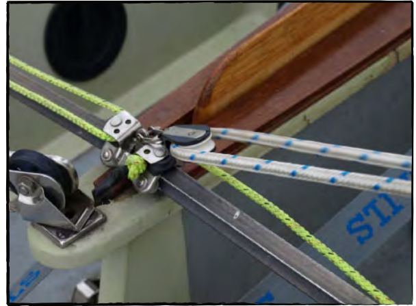
Photo 33, Through the pulley on the traveller
