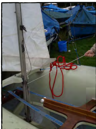
Photo 10, hoist the jib
