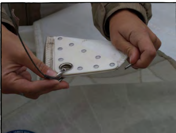
Photo 21, Attach the main sail halyard
