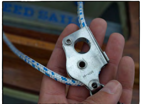
Photo 26, Assemble the kicker
