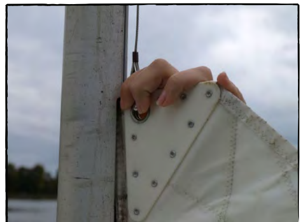
Photo 22, Feed the main sail luff into the mast slot
