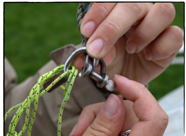
Photo 9, Attach the jib to the halyard
