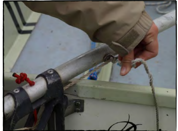
Photo 37, Attach the rudder uphaul
