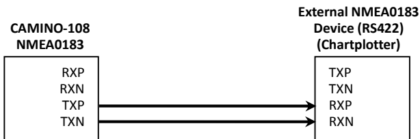
Figure 6 NMEA 0183 Connection illustration
